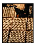
Colt's MAXIM RTO™ Regenerative Thermal Oxidizer is so energy efficient that it can run self- sustaining, without the need for auxiliary fuel, for many industrial applications. The type and quantity of ceramic heat transfer media is specially selected for your application based on the characteristics and chemistry of your processes. Our typical media is structured media (pictured), but random packed saddles and other specialty medias are also available.
